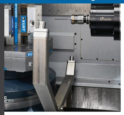
The **Renishaw NC4** and **NC4+** systems allow fast, non-contact tool setting and breakage detection. Available as fixed and separate systems, it can be configured for most machining systems.
