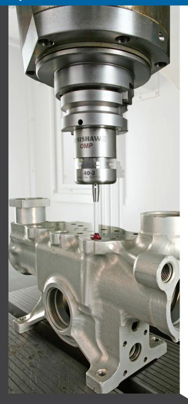
The **Renishaw OMP40-2** features a compact design with optical transmission for small machining centers and machines fitted with small HSK and small taper spindles.
