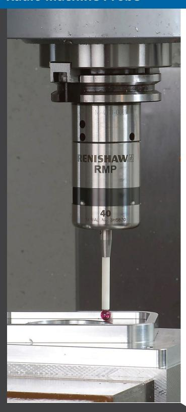
The **Renishaw RMP40** is the ideal choice for multi-tasking applications where the line-of-sight between probe and interface cannot always be maintained.
