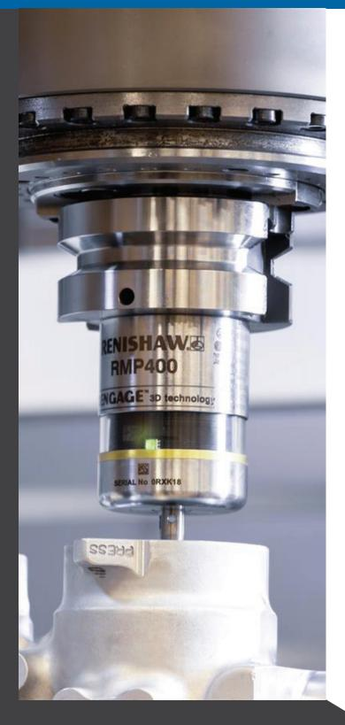
The **Renishaw RMP400** High Accuracy Probe features an ultra compact design with radio signal transmission for small to medium machines.
