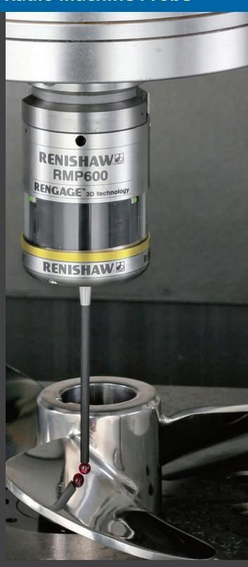
The **Renishaw RMP600** High Accuracy Probe features an ultra compact design with optical radio transmission for medium to large machining and mill-turn centers.
