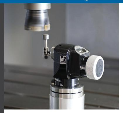
The wireless **Renishaw RTS** is a tool setter with radio transmission suitable for use on machining centers of all sizes, or in applications where line-of-sight between the tool setter and receiver is difficult to achieve.
