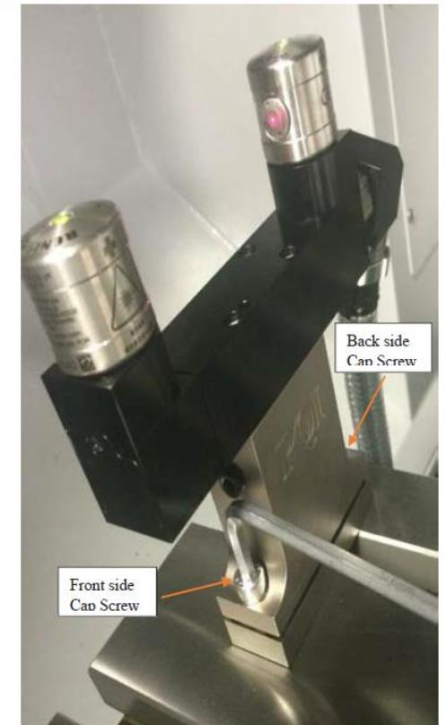
Loosen / Tighten type adjustment.
