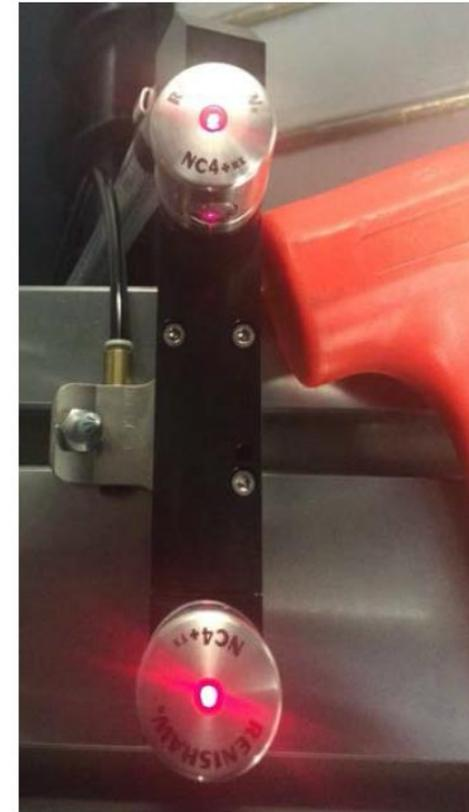
Set screw / Cap screw type adjustment.
