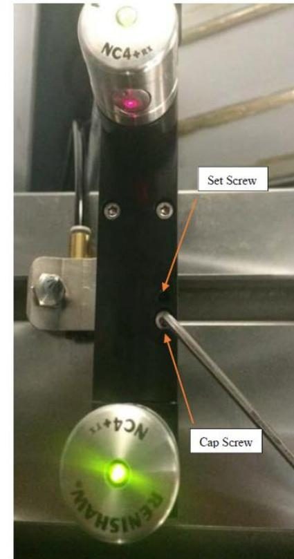
Set screw / Cap screw type adjustment.
