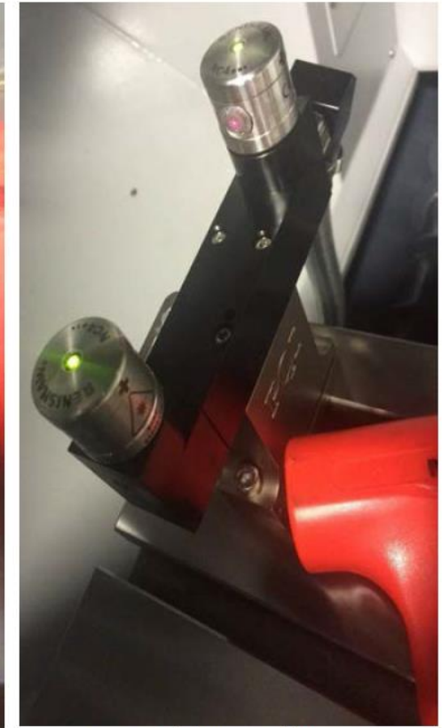
Loosen / Tighten type adjustment. Pqi provided riser mount.
