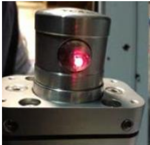
Fig. 3 (The beam is not centered)
